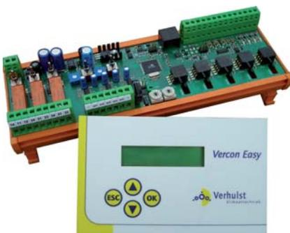
This unit controls the ambient climate within working or living spaces. It directly controls the air conditioning system. A wide variety of control parameters can be modified on the display to fit your requirements. The unit may optionally be connected to a laptop and controlled jointly as a member of a group of network-connected systems.
