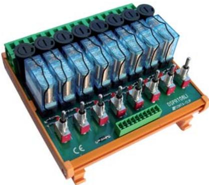
This product was designed to automatically control building blinds and lighting systems. The control system consists of relay and bypass modules that forward signals from a PLC to four groups of eight signals.
