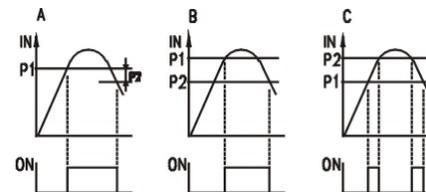
Set the threshold value of potentiometer P1 and P2 by using a screwdriver. Both potentiometers represent a percentage from the selected input value. Full left turn is 0% and full right turn is 100% of the selected input value.
