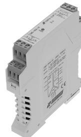
The CMS-I10A-UI is a multi-functional 3-way isolated signal converter. This module is used for galvanic isolated high current measurement and conversion. Also a threshold relay output is provided.
